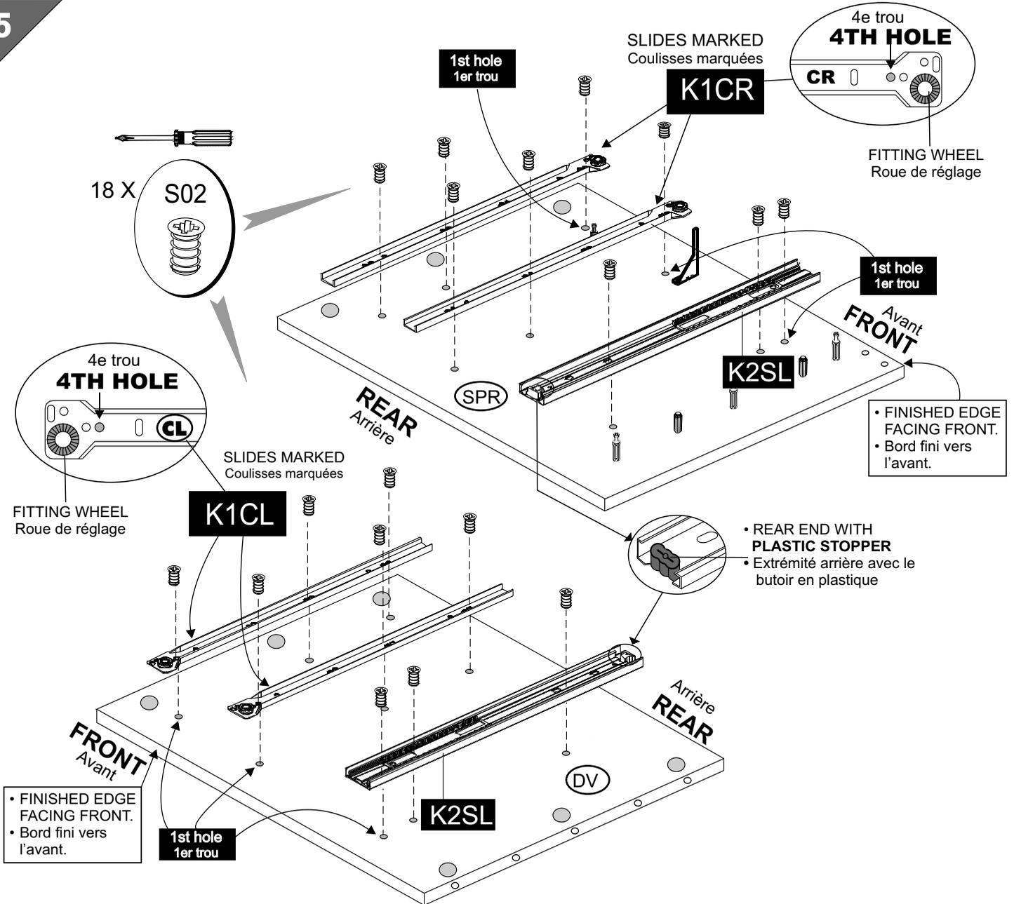
**INSTALLATION OF BOX SLIDE MOUNT CL / CR :**
