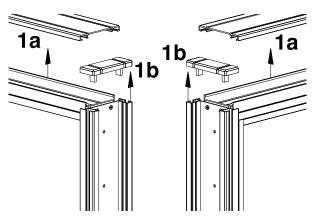
3. Remove all male connecting hooks from the connecting side pillar of one of the two panels.
