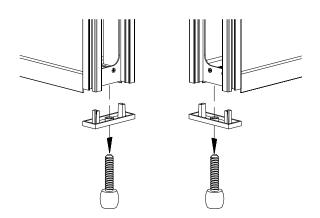
4. Line up the female connecting hooks with holes indicated below. Install one female connecting hook in each instance where a male connection hook was removed. Secure the female connecting hooks with screws removed in Step 3.
