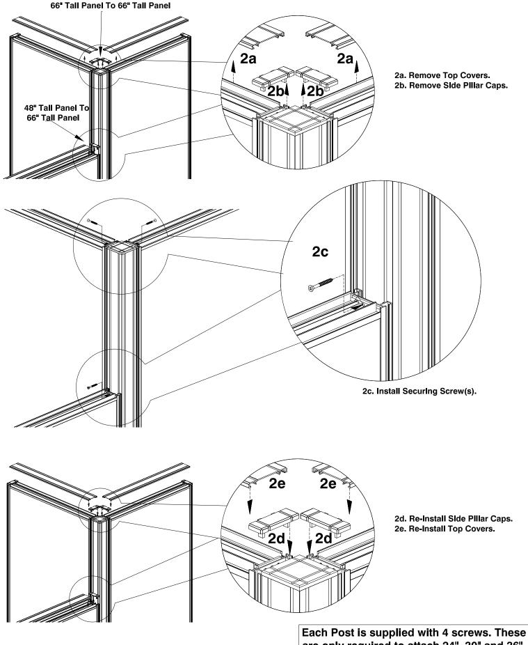
A-2 REV E December 3, 2015 QUESTIONS OR CONCERNS ? PHONE Customer Service 1-800-567-3060 1-250-765-4145 M-F 7am - 4:30 pm PST Each Post is supplied with 4 screws. These are only required to attach 24", 30" and 36" Panels to Posts. Therefore you may not necessarily use all screws supplied.
